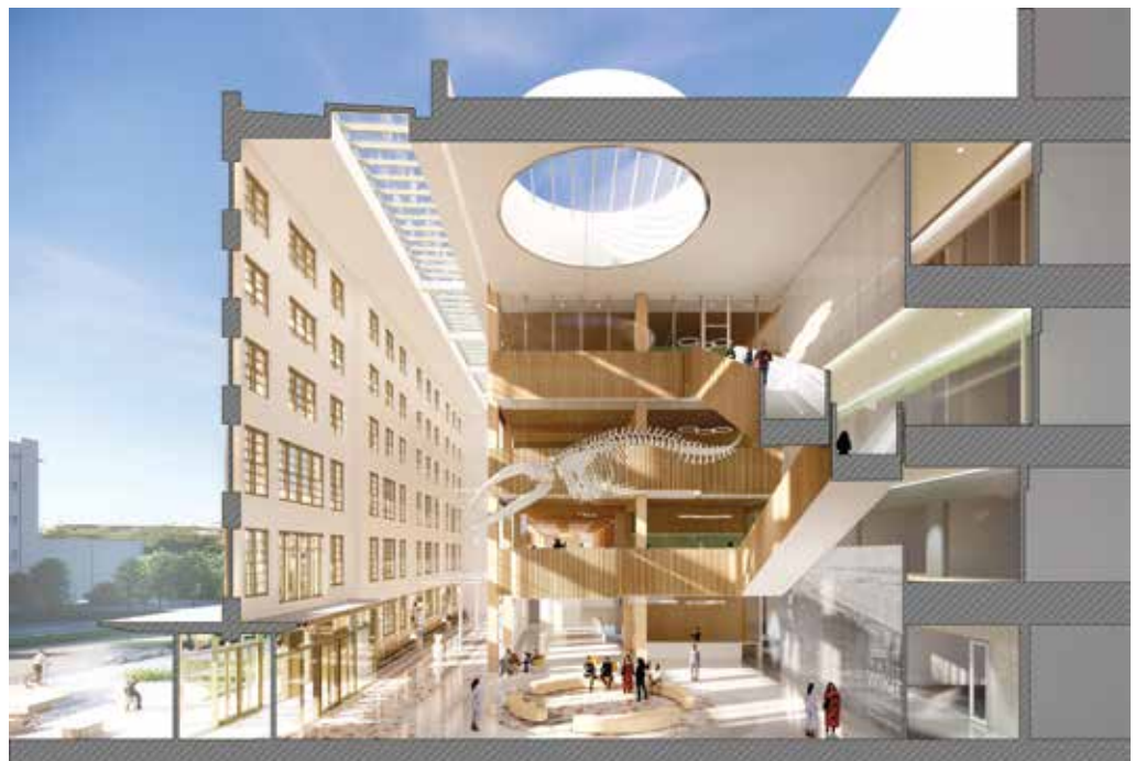
A new roof-mounted skylight will add further daylighting to the atrium, but also into many of the existing adjacent spaces off of the atrium space. Image courtesy of Diamond Schmitt and EXP.
